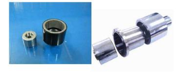
Magnetic coupling is a new kind of coupling, which connects motor and machine by permanent magnetic force. They work in the sealless magnetic drive pumps, which transporting volatile, flammable, explosive and toxic solutions with no leakage.
